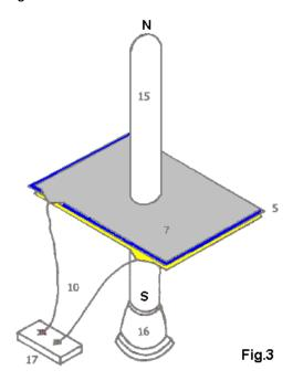
**Fig.3** is a Proof Of Principal Device using a Plasma Tube as an active Dipole. In this drawing, **5** is the plastic sheet dielectric separator of the two plates **7** of the capacitor, the upper plate being aluminium and the lower plate copper. The connecting wires are marked **10** and the plasma tube is designated **15**. The plasma tube is four feet long (1.22 m) and six inches (100 mm) in diameter. The high-voltage energy source
