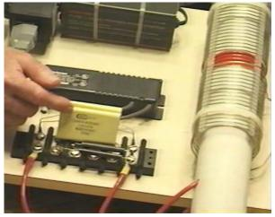
The L1 / L2 coil arrangement is a Tesla Coil. The positioning of the "L1" coil along the length of the "L2" coil, adjusts the voltage to current ratio produced by the coil. When the "L1" coil is near the middle of the "L2" coil, then the amplified voltage and amplified current are roughly the same. However, Don stresses that the "height" length of the coil (when standing vertically) controls the voltage produced while the coil "width" (the diameter of the turns) controls the current produced.
