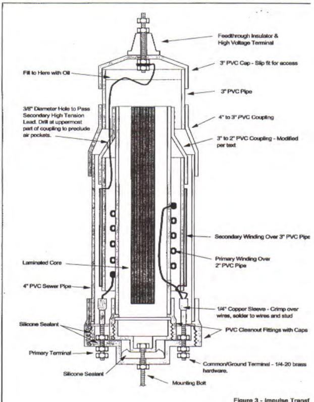
Figure 3 - Impulse Transf Assembly (Note, vertical : shortened.)
