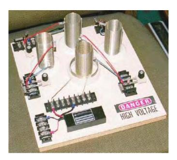
The coil in the centre of the board is a power transmitter made from a Tesla Coil constructed from two Barker & Williamson ready-made coils. Three more of the inner coil are also used as power receivers. The outer, larger diameter coil is a few turns taken from one of their standard coils and organised so that the coil wire length is one quarter of the coil wire length of the inner coil ("L2").
