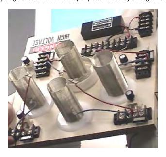
The "L1" short outer coil is held in a raised position by the section of white plastic pipe in order to position it correctly relative to the smaller diameter "L2" secondary coil. Again, it appears to have five turns:
