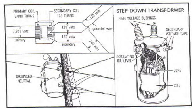
Single Phase - The most common type of electrical service or power available to consumers. One transformer is used between the distribution line and the meter. Usually three wires, two "hot" and one neutral, are installed to provide 120V and 240V single-phase service. Single-phase service may also be supplied with three-phase service.
