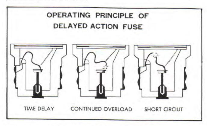
Fustats, nontamperable fuses of the time-delay type, have a different size base and require a special adapter that is screwed into the standard fuse socket. After the adapter is installed, it cannot be removed. For example, the installation of a 15-ampere adapter allows only the use of 15-ampere or smaller fuses.
