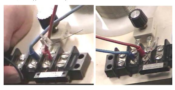
As there are very slight differences in the manufactured coils, each one is tuned to the exact transmitter frequency and a miniature neon is used to show when the tuning has been set correctly.
